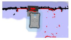
Figure 5.1. The red laser scanner line along a wall indicates that the robot is localized correctly in an active map.
