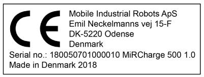
Figure 4.2. Example of MiRCharge 500 CE marking and identification label
